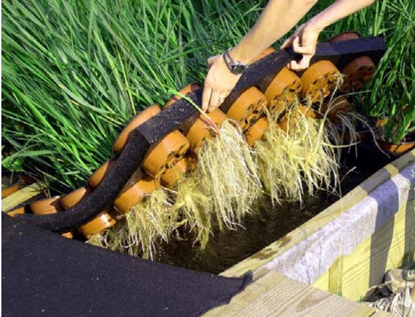
View of floating wetland raft system exposing root growth.
