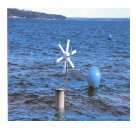
The steel spar buoy deployed with a Rutland 913 Wind Charger.
