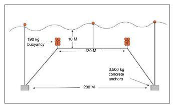
Figure 2. Diagrammatic representation of a submerged longline system used in offshore waters in New Hampshire. Diagram courtesy of Richard Langan, University of New Hampshire.
