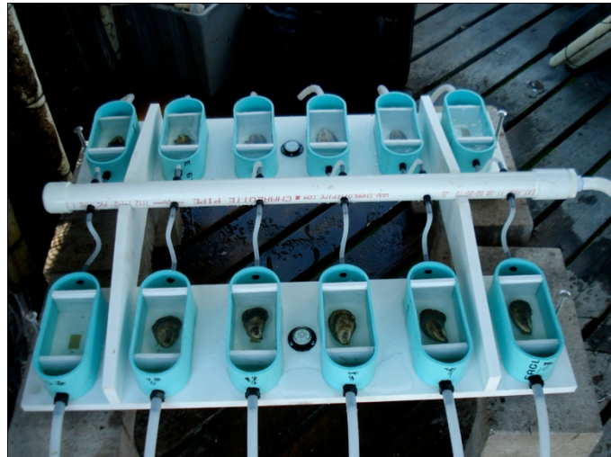
Figure 3. Flow through feeding manifold with 10 oysters and 2 control chambers.
